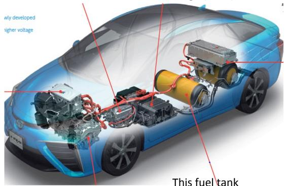
out of the two used in the Mirai may not be required at all (-60L)
