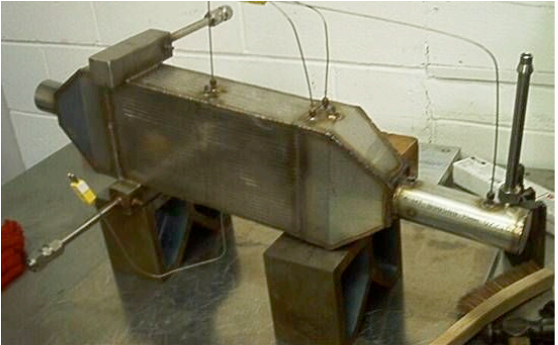
Analytic Power -All Brazed, Iron Catalyzed, 5kW Cracker
