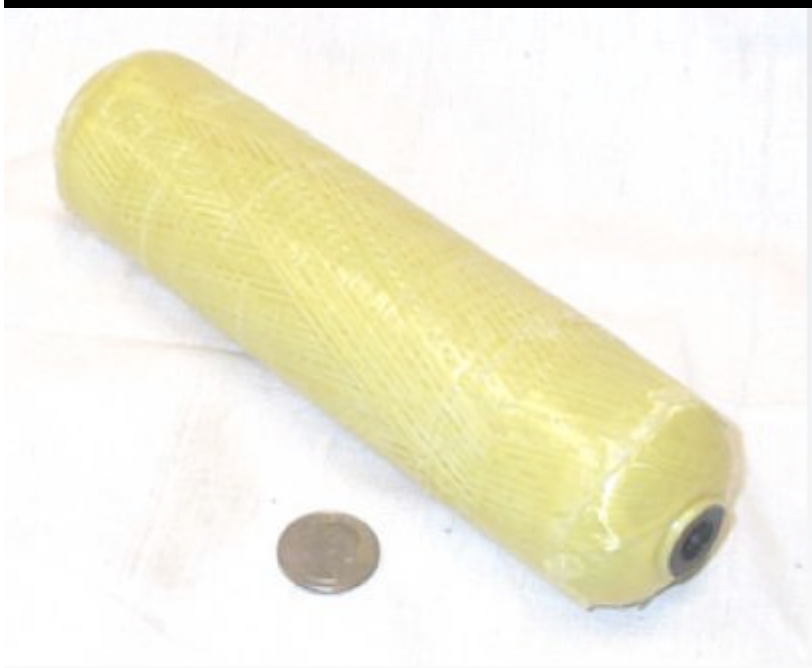
Fiber-composite tank formed with safe-storage material
