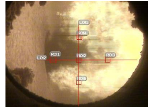
Flame at the outlet of burner 20% ammonia co-firing
