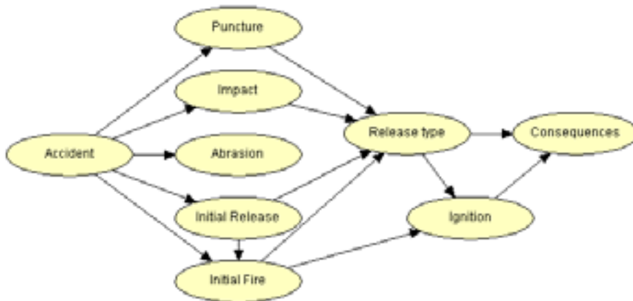
Figure 1 Bayesian net describing the conditional probabilities of dangerous consequences of an accident with an LPG road tanker.
