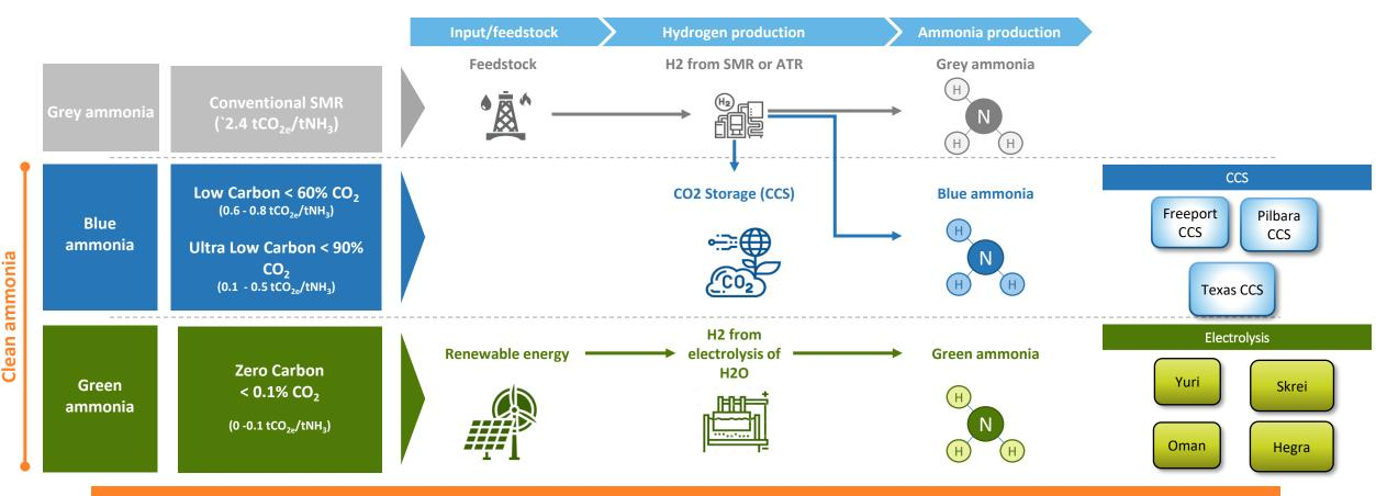
The Haber-Bosch process is used to synthesize ammonia from hydrogen, producing an identical ammonia molecule regardless of "color"
