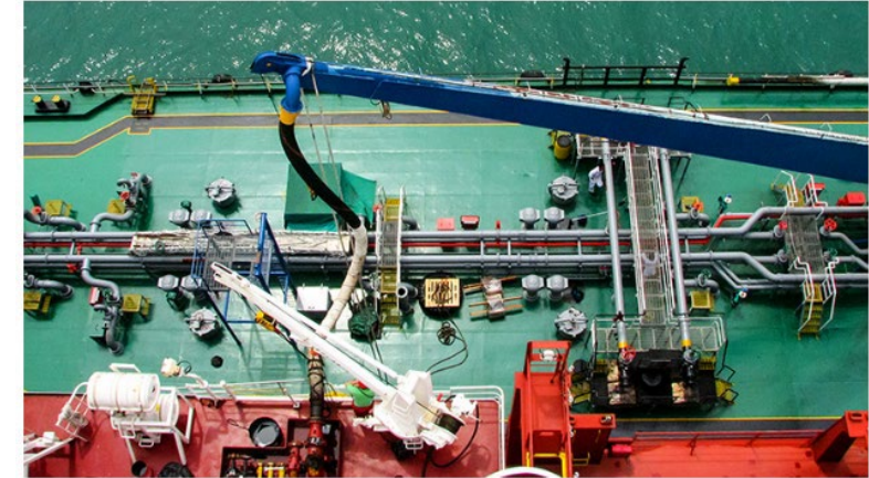
Powered Emergency Release Coupler (PERC) for cryogenic gas
