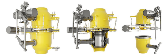
Key principles of PERC: synchronized closure of ball valves (to isolate inventory) before parting
