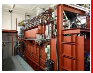
May 2023 J-Engine commenced NH3 combustion test in the test rig of the 2-stroke engine
