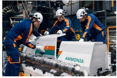
Gas admission valve on cylinder head -unit
