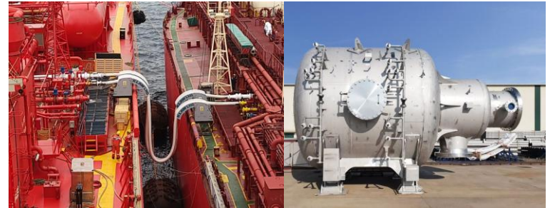
Top: Fuel Supply System, Ammonia Release Mitigation System, DeNO x (Wärtsilä). Bottom Left: Ship-to-Ship bunkering (GCMD). Bottom Right: DeNO x system (BUTTING).
