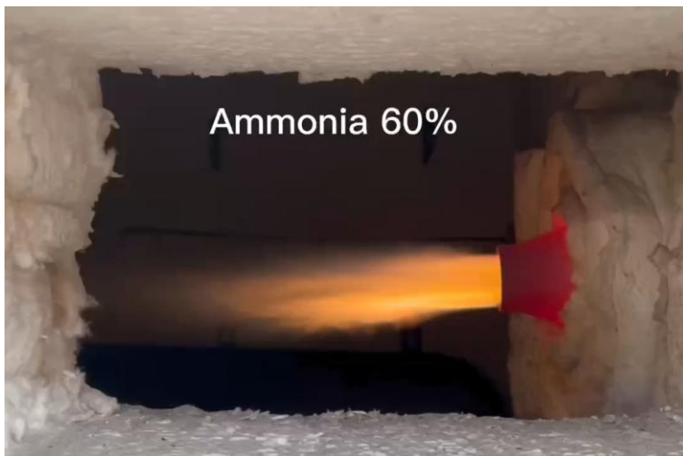
Combustion of ammonia-natural gases in industrial burners
