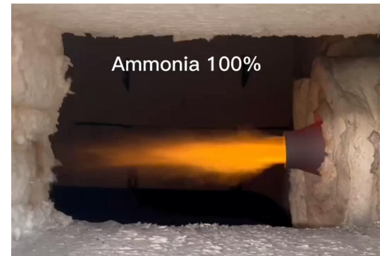
Combustion of ammonia-natural gases in industrial burners
