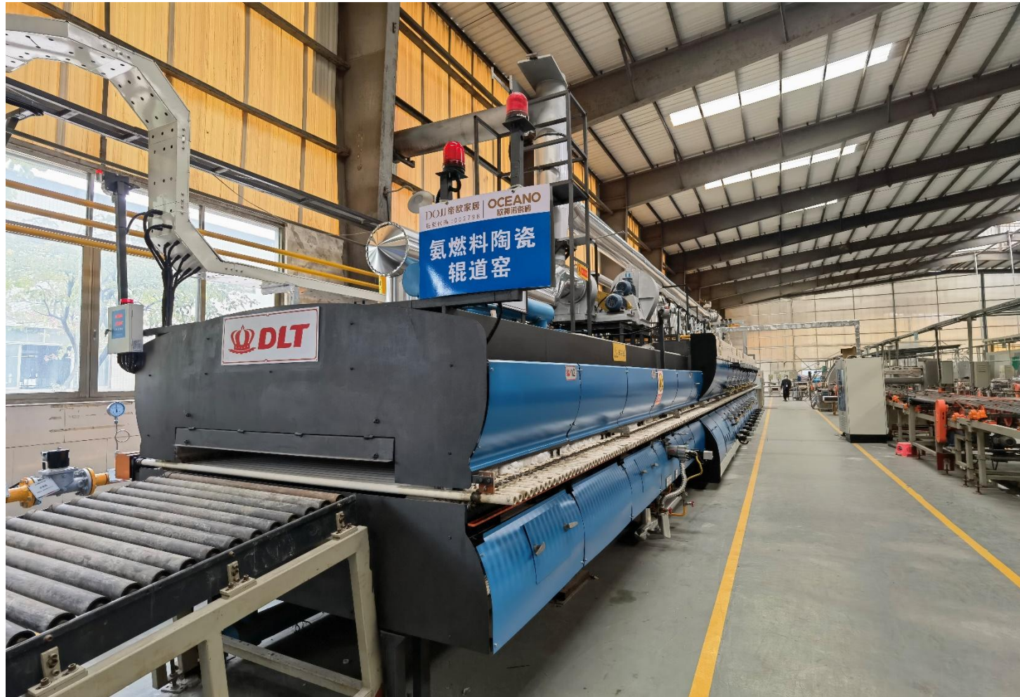
Pilot ceramic roller kiln of 30m long, at the Oceano Ceramics Co., Ltd, ceramic tile production capacity of 100,000 m 2 /year
