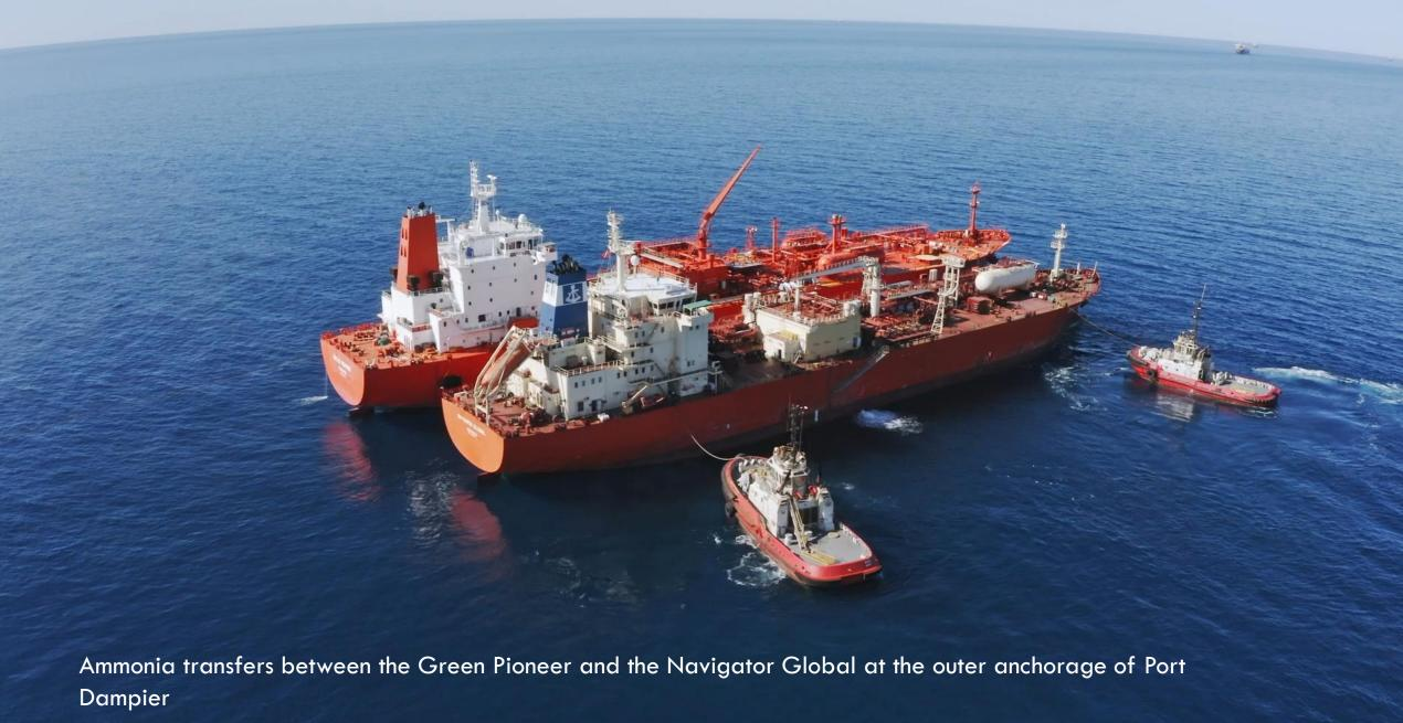
4,000 m<sup>3</sup> (2,700 MT) of liquid ammonia was transferred at 700-800 m<sup>3</sup>/h from the Green Pioneer to the Navigator Global and back
